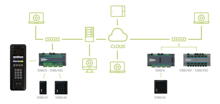
The 2 Smart controller manages 4 gates with the possibility of adding an expansion module for another 2 gates, while the Wiegand controller manages 2 gates without expansion module and 6 gates with expansion module. The controllers can be powered via PoE or with local 12Vdc power supply.
