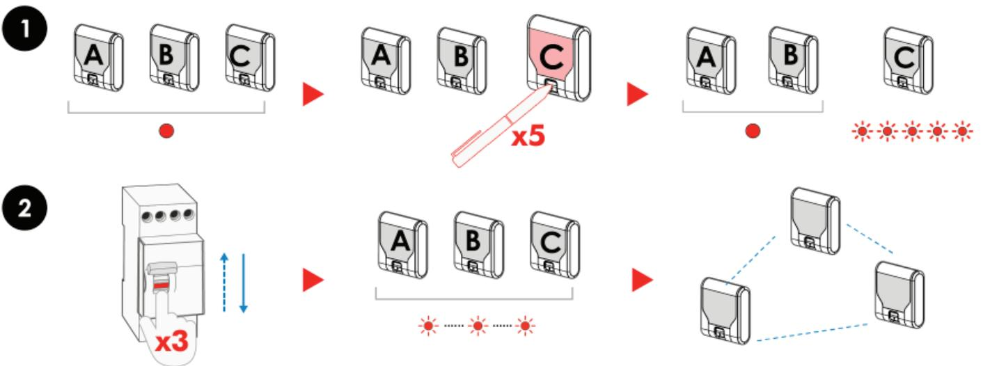
NB: Connection to the receiver network can take between 5 and 20 seconds
